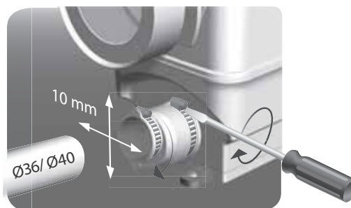
Fig. 35 Height and side alignment possible when using Ø36/40 inlet pipes
